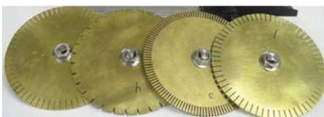
Figure 4 Mechanical chopper wheels for use in time-resolved single-crystal experiments.
